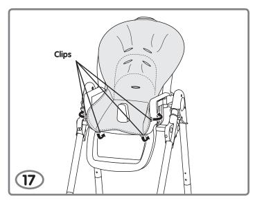
• Fit the clips on the front edge of the pad onto the seat bottom.
